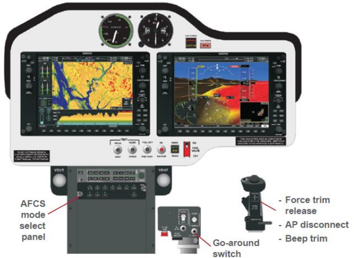
Bell 407GXP Flight Deck with Autopilot.
